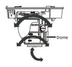
8. When you adjust the camera vertically, loosen the fixing screws on both sides lightly, rotate the camera to the desired monitoring direction and then fasten the screws. Please stop rotating the camera when the spacing point is blocked, otherwise the camera lens might be damaged.
